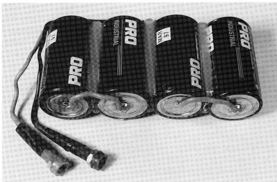
Duracells glued together with sealant.
